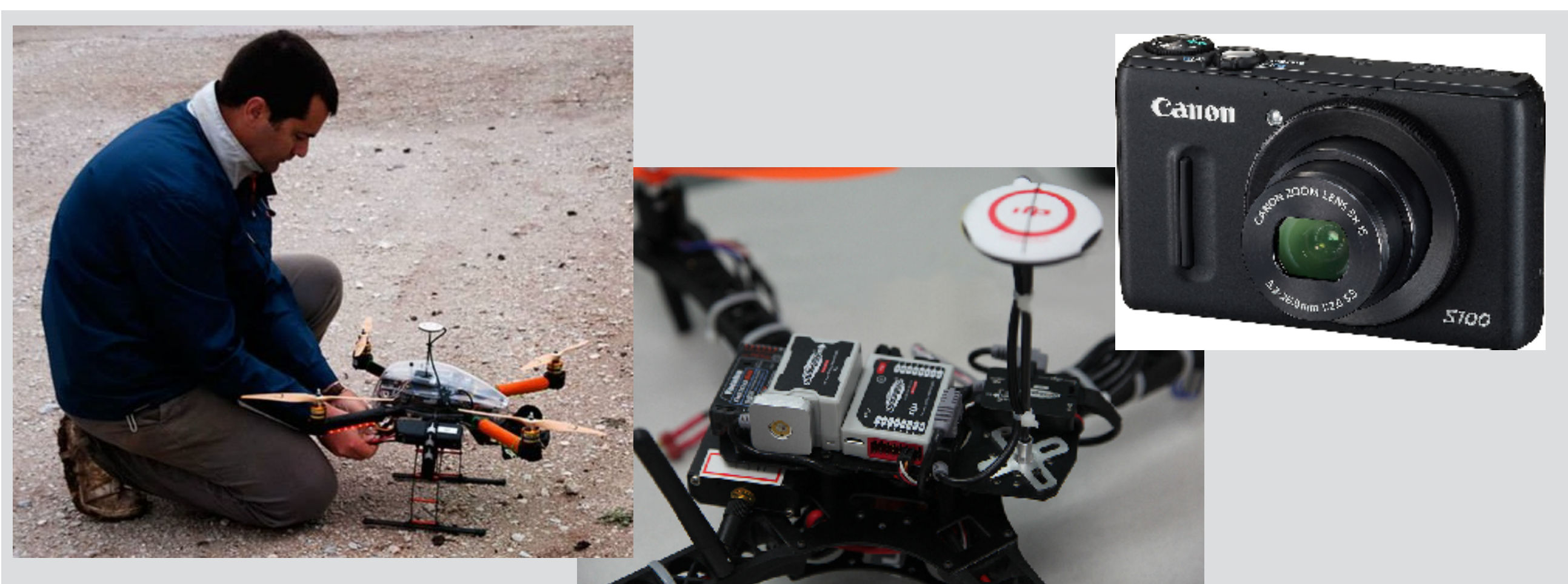
Fig2. Basic equipment for the field (UAV) campaign: the CX4 Droidworx, DJI navigation system and the compact camera.
